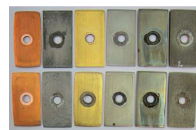
Stat. Corrosion acc. ASTM D 1384 Test concentration: 1,5 % v/v Protectogen C aqua in ASTM water Test duration: 1000 hours
