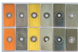
Stat. Corrosion acc. ASTM D 1384 Test concentration: 1,5 % v/v Protectogen C aqua in ASTM water Test duration: 336 hours
